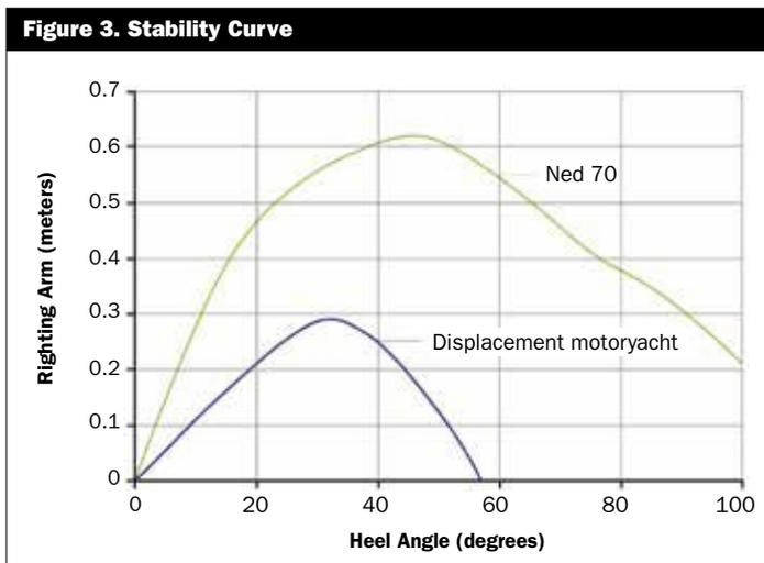
providing stability for ocean passages. So the Ned 70 is a long and slender yacht, which can clearly be seen in the length-to-beam ratio as indicated in **Figure 2**. But even with this slender hull shape, the stability is still excellent, as illustrated in **Figure 3**.
