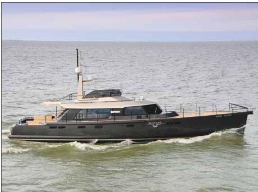
At cruising speed the Ned 70 moves through the water with little fuss. Her Froude number at that speed is just 0.325, which means she expends very little energy to overcome wavemaking resistance.
