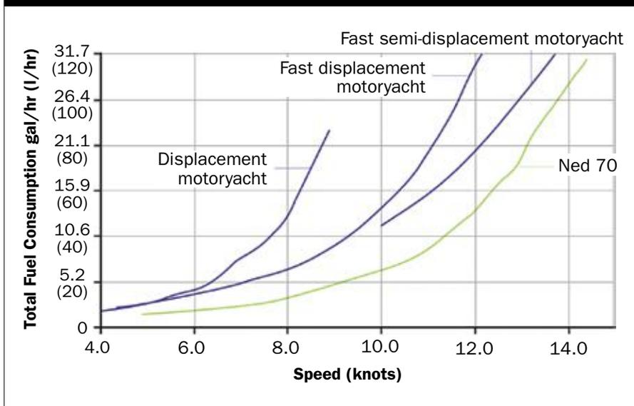
The low resistance of the LDL hull minimizes power needs at displacement speeds, which starts a virtuous spiral requiring a smaller, lighter-weight propulsion engine and reduced fuel capacity to match the comparatively modest burn rate.
