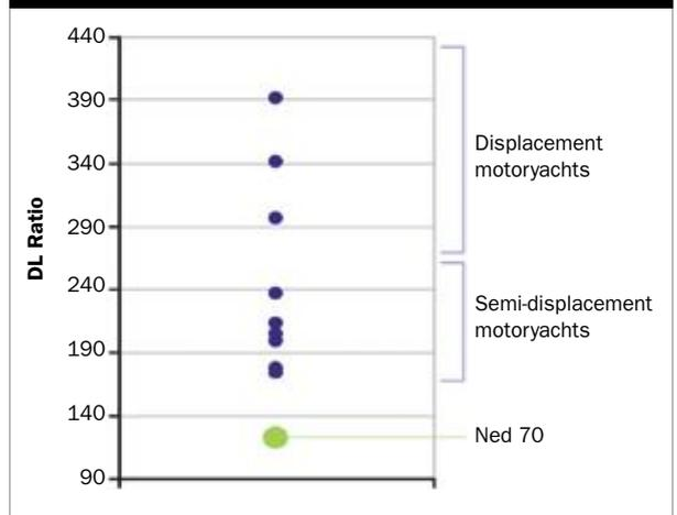
*Ned 70 stacks up well against more conventionally efficient semi-displacement powerboats. The specified design goal of minimizing the displacement/length ratio helps the designer keep the overall weight of the vessel low even in the face of temptations to add heavy accommodation or powering options.*
